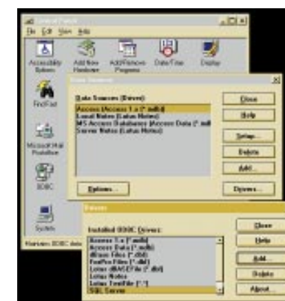
If ODBC is installed on your computer, you need to install an ODBC driver in the Windows Control Panel for each database type you wish to open
